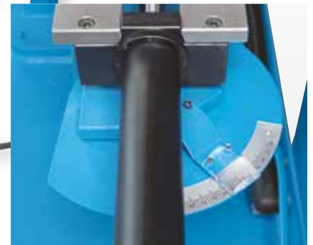
The cutting angle is precisely adjustable and can be easily read
