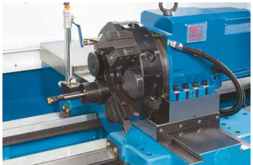
VDI 30 tool turret with 8 stations
