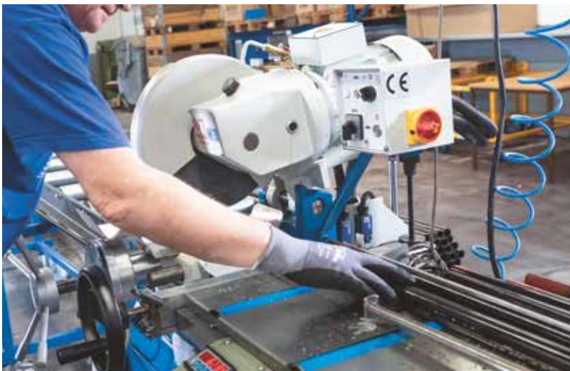
The preliminary work at Minimax is done by the KHK 350 semi-automatic circular saw with pneumatic workpiece clamping, also from KNUTH. It brings the steel pipes exactly to the correct length.
