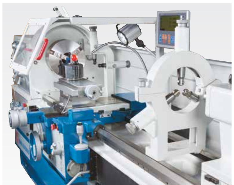
Rests ensure maximum precision when machining long workpieces
