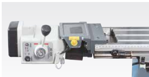
Infinitely variable milling table feed
