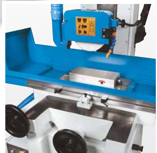
Permanent magnetic clamping plates with micro pole pitch - ideal for high-precision grinding work
