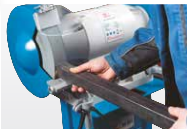
Rigid, wide material support ensures operator safety
