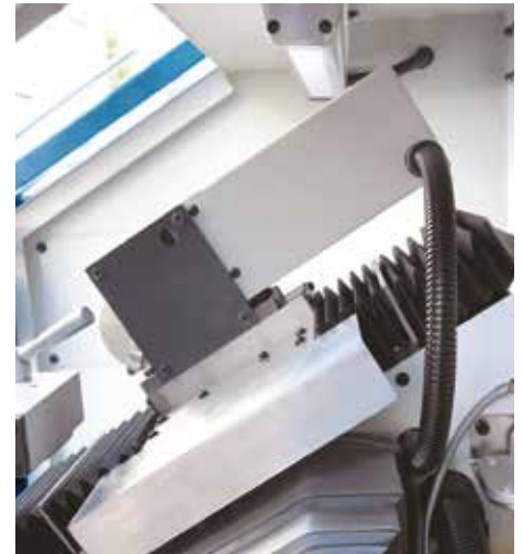
Inclined bed design optimizes work space and chip removal
