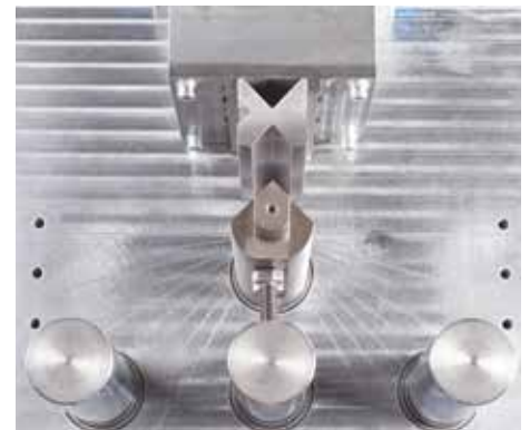
Angle lines are engraved in the work table for easy orientation
