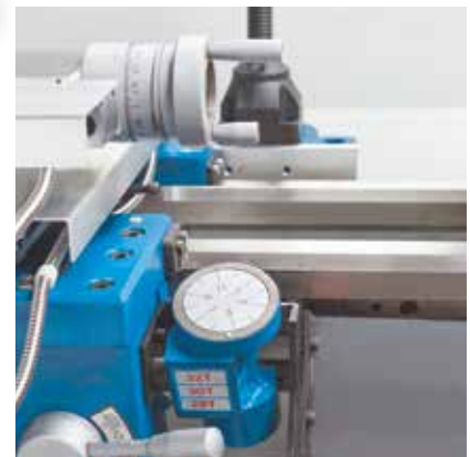
The thread gauge allows for resuming the thread
