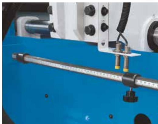
Automatic workpiece feed and traversing vise with manually adjustable stroke limit stop
