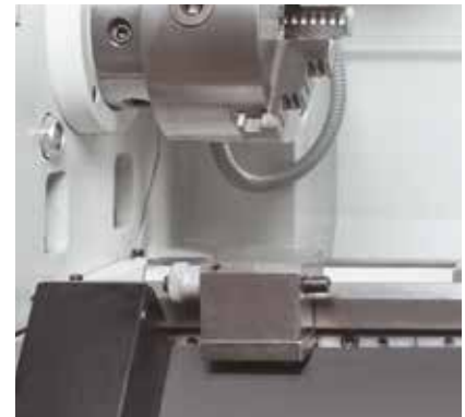
Micrometer bed stop ensures repeatability
