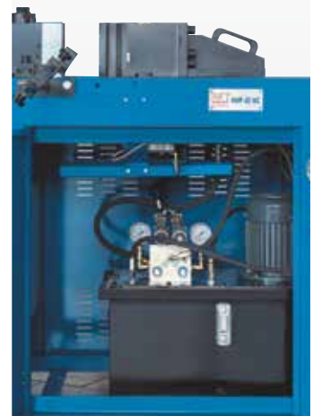
Compact hydraulic unit located accessibly inside the base
