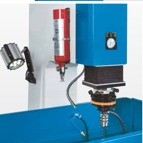
Fire extinguishing system for added safety
