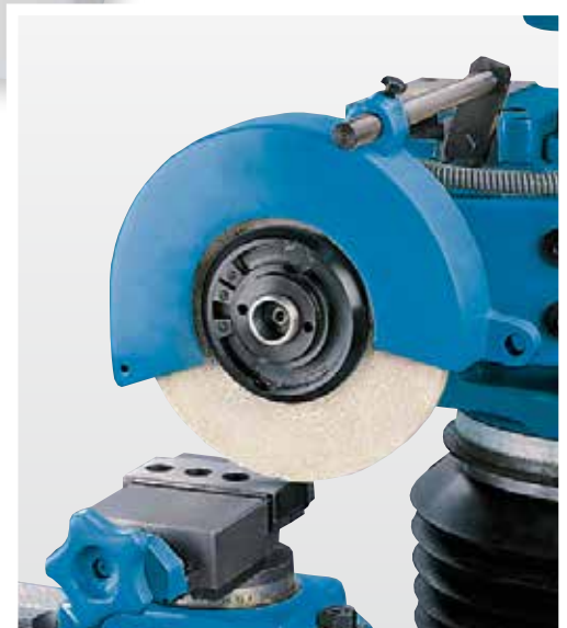
Surface grinding with angle-adjustable vise
