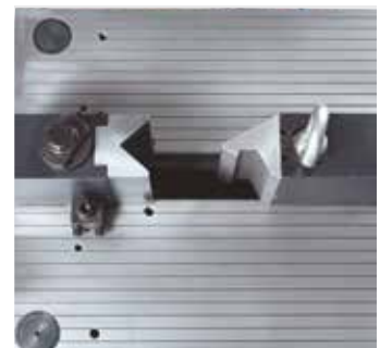
Long, supporting, hardened bending die guideways with central lubrication system
