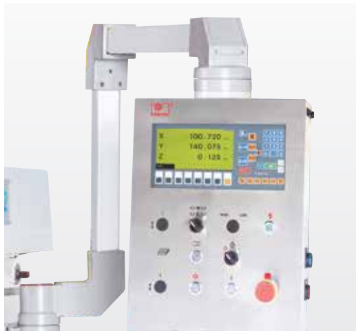
Swiveling control panel with integrated position indicator for maximum operator comfort
