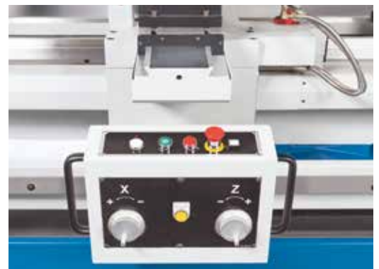
Compact control unit with electronic hand-wheels
