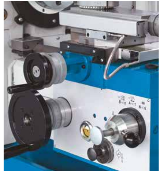
Central lubrication is integrated into the support for easy maintenance and handling
