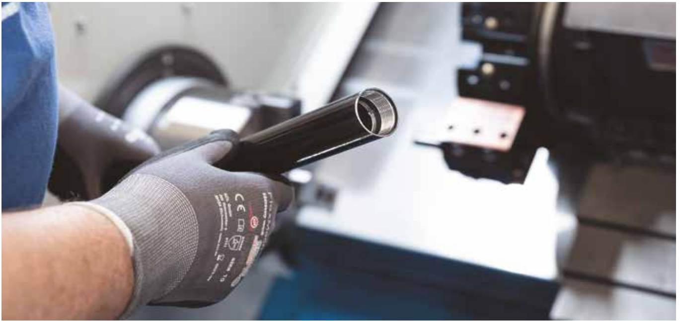
The highest precision is required when turning the thread. The steel pipes are later precisely connected to form lines for dry sprinkler systems.
