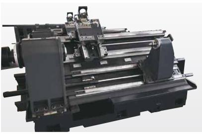
The programmable hydraulic tailstock can be positioned along the entire machining length
