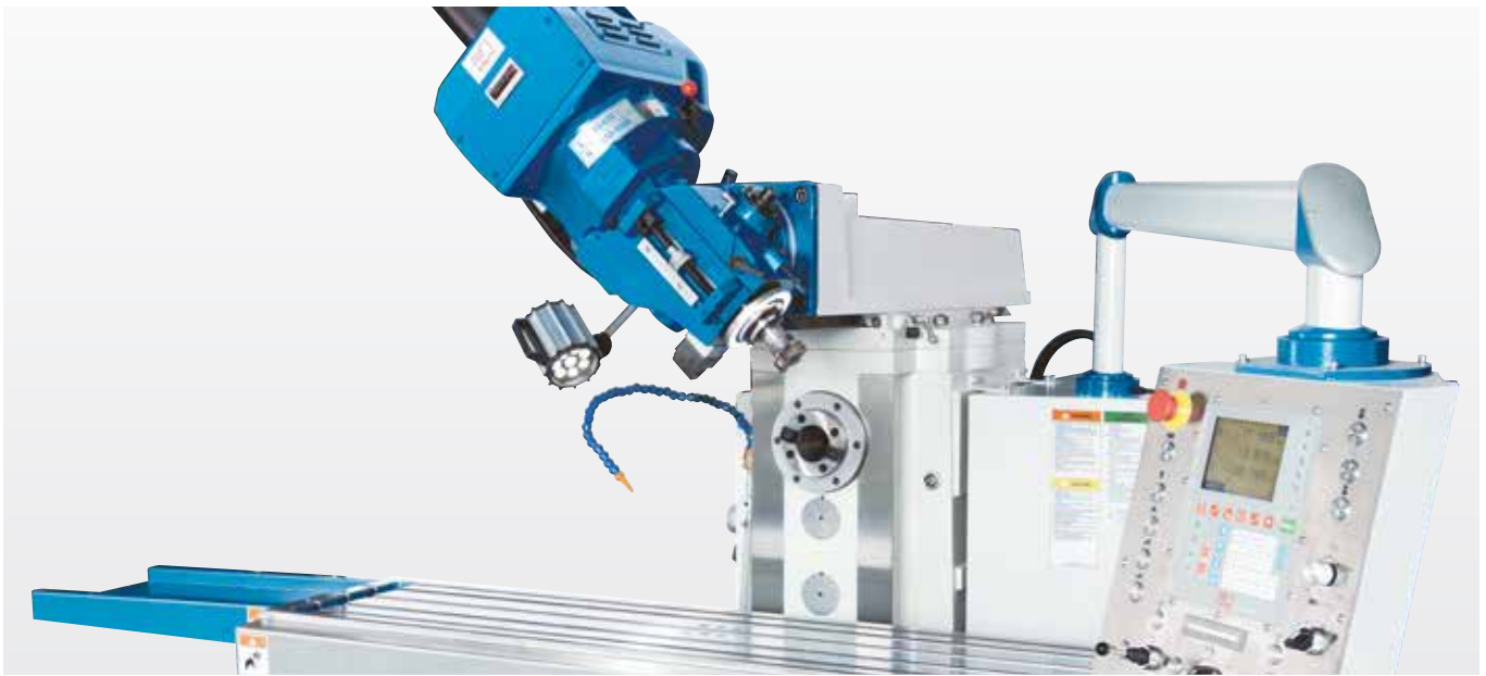
Cutter head swivels 45°
