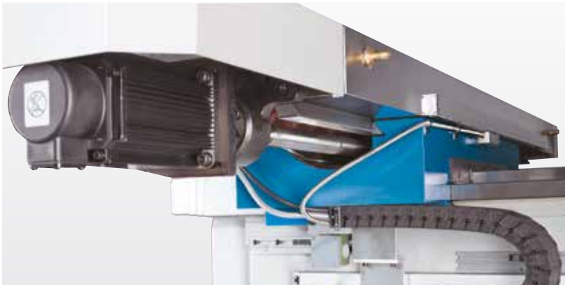
Preloaded ball screws ensure high precision
