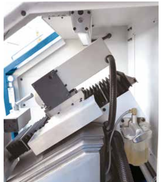
Inclined bed design optimizes work space and chip removal
