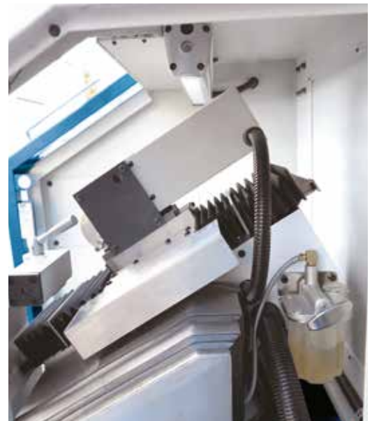
Inclined bed design optimizes work space and chip removal
