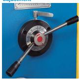
Facilitates quality cutting for a wide range of plate thicknesses by adjusting the gap distance.
