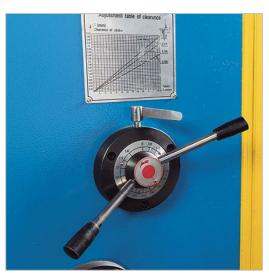
Based on the sheet thickness, to improve the cutting quality the gap between the blades can be easily set using the adjusting system from the machine side.
