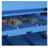
Using the pneumatically controlled sheet metal holding device, even thin metal sheets can be positioned exactly on the backgauge.
