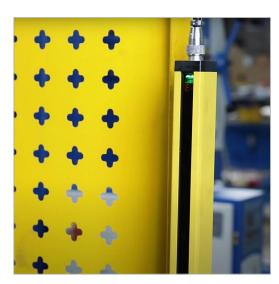
On the back-side, a light barrier from LNTECH is installed to secure the working area of the back gauge.
