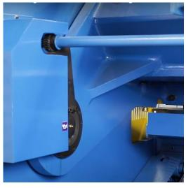
Using a swing beam design, the top knife holder is curved and it follows an arched motion around a lever support, offering a precise cut.
