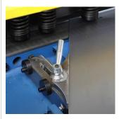
Easy to use angle stop with clamping lever and angle scale.
