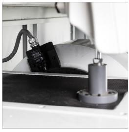
Additionally, a spindle cover is provided to protect the operator. It integrates an interlock system, stopping the spindle when to cover is lifted
