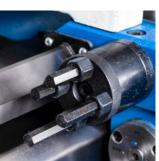
Turret stop with 4 positions which are used as spacers when paired with a micrometer stop
