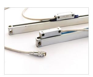
Optical Scales: 5 micron resolution (0.005 mm) with outside cover from aluminum for protection against oil, coolant and chips
