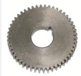
Change gears for thread cutting
