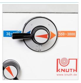
The frequency inverter reduces the number of speeds to only two, with infinitely variable speed adjustment
