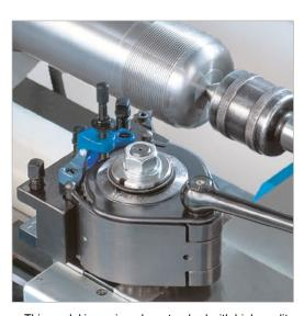
This model is equipped as standard with high quality German type quick change tool post to easily switch the tools with repeat accuracy of 0,01 mm
