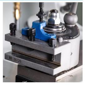
• Lathe knives are easily clamped using thumb screws
