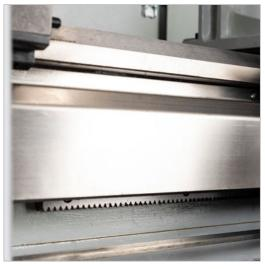
The leadscrew has a steel cover which on one side is shielding it from falling chips and in the same time assures maximum safety for the operator
