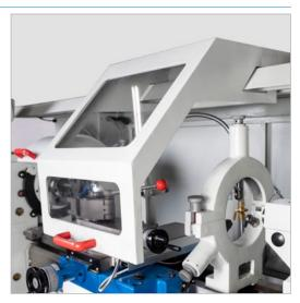
For extra protection against chips and coolant splashes, a large liftable cover is installed over the toolpost which travels together with the carriage
