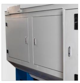
The new cover design includes two large side doors which facilitates the mounting of complex workpieces and maintenance
