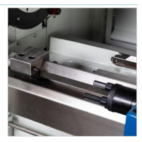
Machine is equipped with micrometer and turret stops for precise operations
