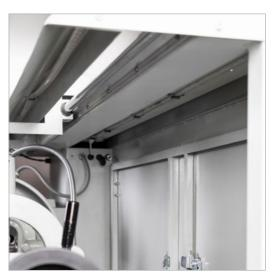
Work light is provided along entire work area through industrial LED light bars which are integrated in the machine cover
