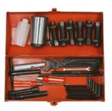
Tool box with tools for operating the lathe and maintenance
