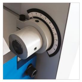
Setting the required bending angle is easily done with the adjustable angle stop from 0° and up to 135°
