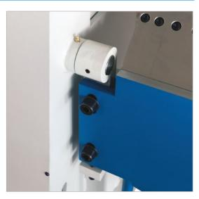
These models are designed with side screws for easy adjustment of the distance between top and folding beam, according to sheet thickness
