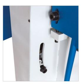
Clamping adjustment is done using the screws situated on internal side of machine feet
