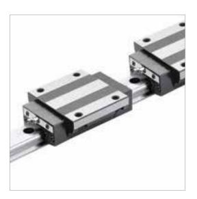
Special linear guide ways from HIWIN on all axes, designed for large load capacity with high rigidity. They feature equal load ratings in the radial, reverse radial and lateral directions, and are selfaligning to absorb installation-error. They are designed for long life and smooth linear motion even at high speeds.
