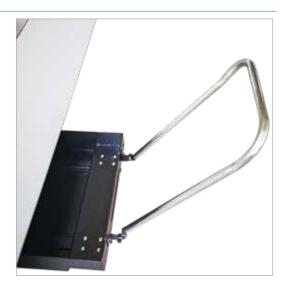
Machine is equipped standard with lateral scrap drawers which allow the removal of small sized parts and waste material without interrupting the cutting process.
