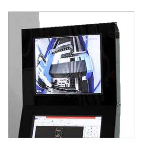
You can have full visualization of the cutting process through two cameras which provide complete real time monitoring of operations. One is inside the housing, targeted on the cutting process and the second one is in the back, for checking the table exchange system.
