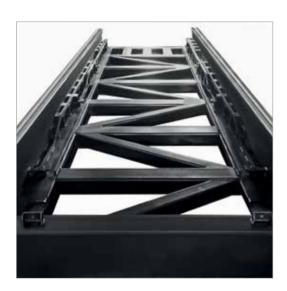
A thermal treatment is applied to the welded machine frame and all structural parts. This eliminates all production-related material stresses – ensuring long-lasting, precise alignment of all components.
