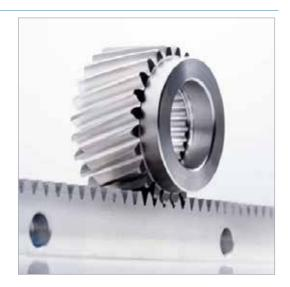
The transmission on X and Y axes is done using high quality helical rack and pinion from the Taiwanese supplier - KAI HE. This low-wear and low maintenance drive system easily handles heavy load capacities and duty cycles due to a higher contact ratio (number of effective teeth engaged).
