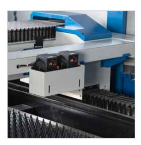
All guideways and racks are fully covered with high quality bellows, which protects against premature wear, while keeping away dust, slag and small cut parts.
