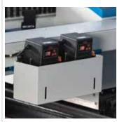
Mounted behind the bridge, this unit ensures automatic central lubrication, which minimizes service requirements and greatly increases machine reliability.
