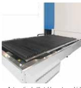
Automatic shuttle table system which minimizes production downtime using the second table for setting the plates or unloading the cut parts, during the cutting process.
