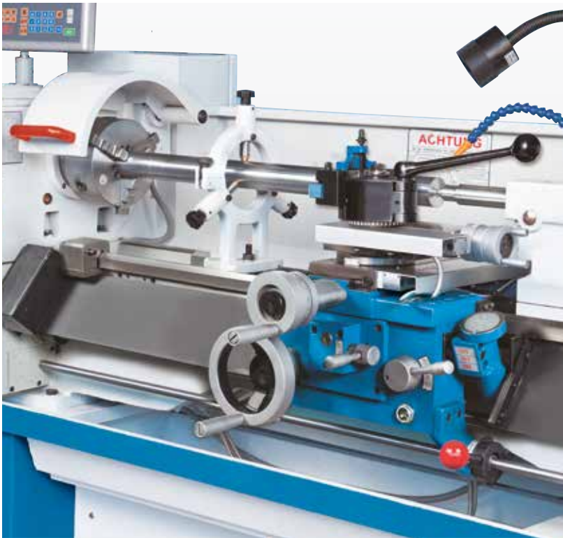
Long workpieces are supported in rigid rests
