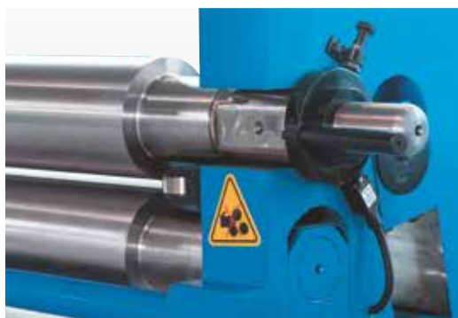
Upper roller can be swiveled out
