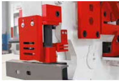
Notching station with safeguard
