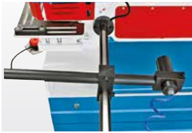
Back gauge with automatic cut activation
