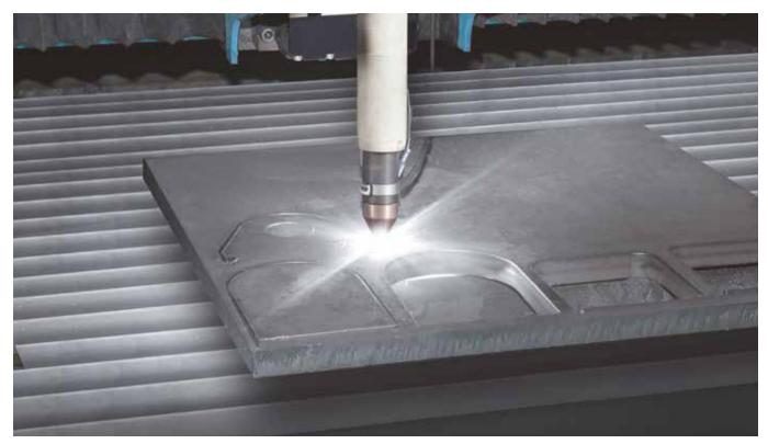
In plasma cutting, the electric arc between electrode and workpiece is constricted by a cutting nozzle so that a plasma beam of high energy density is generated as an effective cutting tool for metals.
