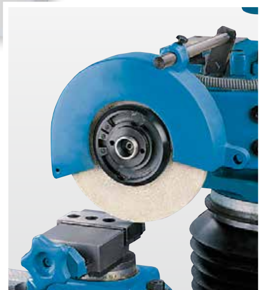
Surface grinding with angle-adjustable vise
