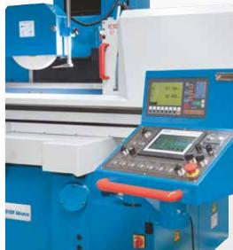
If set to Auto mode, the user-defined roughing and finishing parameters, number of spark-out strokes, and return to zero are automatically processed
