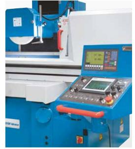
If set to Auto mode, the user-defined roughing and finishing parameters, number of spark-out strokes, and return to zero are automatically processed
