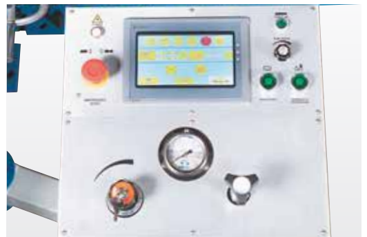
Control panel with graphic touchscreen display
