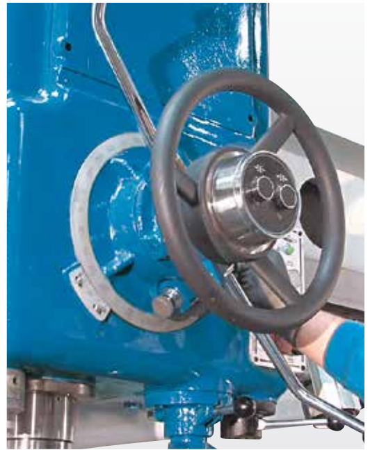
Depth stop with vernier scale
