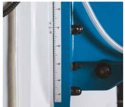
The very rigid cutter head can be precisely swiveled and aligned
