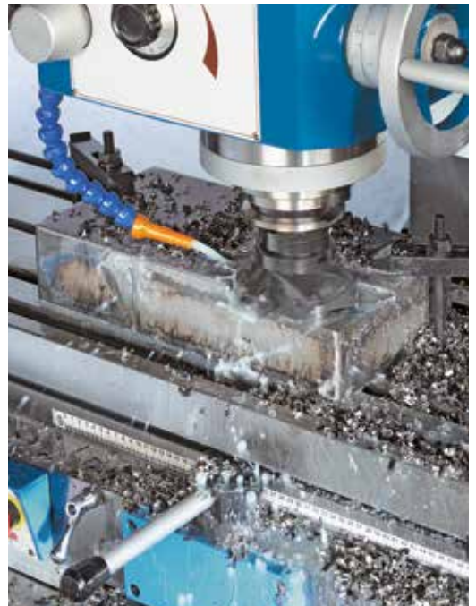
Face milling with measuring head
