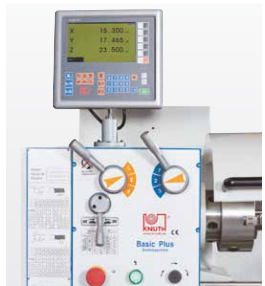
Positioning indicator on X, Z and Z1 axis
