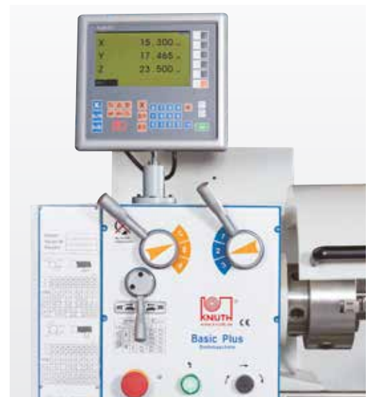
Positioning indicator on X, Z and Z1 axis
