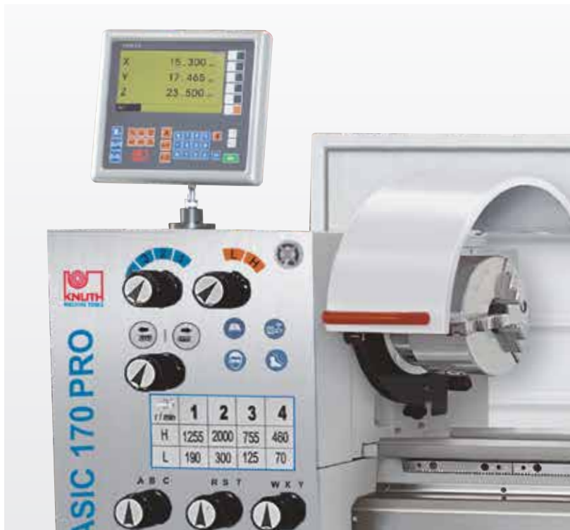
Position indicator on X-, Z- and Z1-axis
