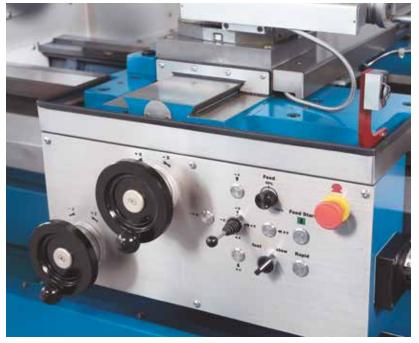
Operation via electronic handwheels in the  $\boldsymbol{\mu}$  range - in feel and position as with a conventional machine
