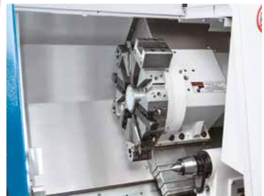
Servo-turret of an Orion 10 TL
