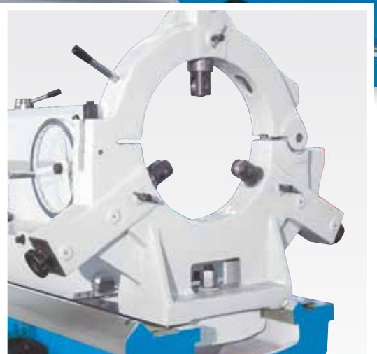
Steady rest with large capacity
